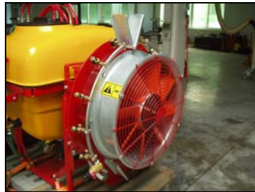
Fig. 13: Axial fan with 1 gear and adjustable fan blades and deflecting equipment
