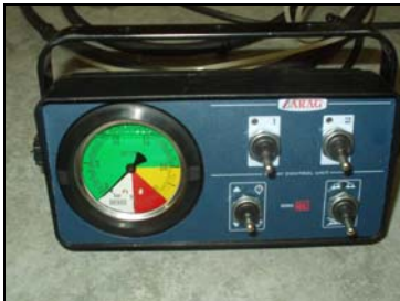
Fig.10: Spray control unit
