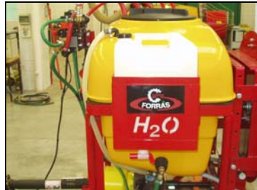
Fig.8: Clean water tank
