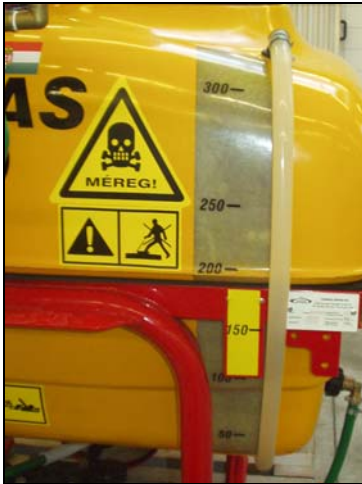
Fig.5: Tank contents indicator
